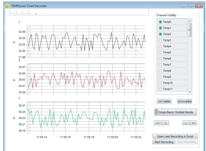
Created with Measure Foundry, the TEMPpoint application allows you to acquire temperature data and then view, graph, or log the data to disk. It can be customized using Measure Foundry to meet any application need.
