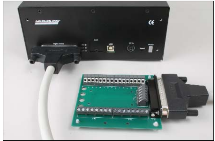
Figure 15. Digital inputs and outputs are easily connected via the 37-pin D-sub connector on the back of the instrument using the STP-37 screw terminal panel and 37-pin EP333 cable.
